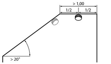
Fig. 17 Straight mounting surface at least 1 m long and 1 m wide
